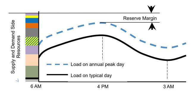
Figure 5.2 – Illustration of Load Curve and Planning Reserve Margin
